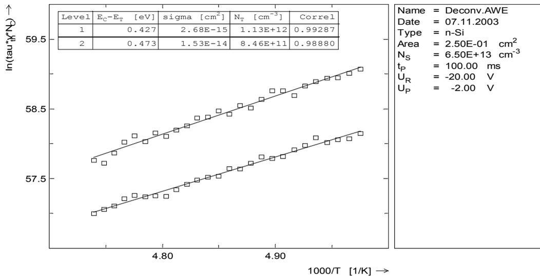
2. Deconvolution of period width scans (similar to frequency or rate window scans)
