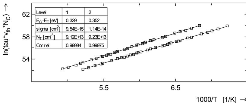
Arrhenius plot from the above tempscan using several measurement files and all (28 per file) correlation functions.
