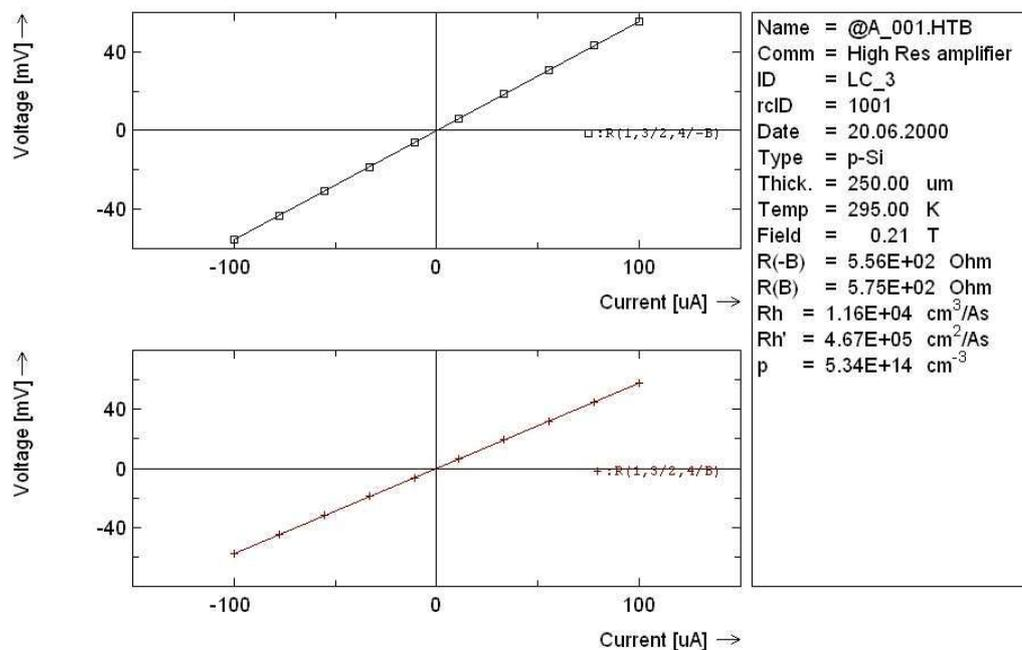
The Hall coefficient  $R_H$  can also be measured using more than 2 B-fields by measuring the Hall resistance as a function of the magnetic field.  $R_H$  can be calculated then from the slope of the  $R(1,3/2,4,B)$  versus B plot by:
