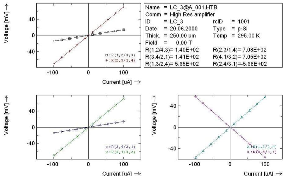
Using these definitions and the results of van der Pauw (Philips Res. Rep. 3 1958) the specific resistivity can be calculated out of two 4-point measurements:
