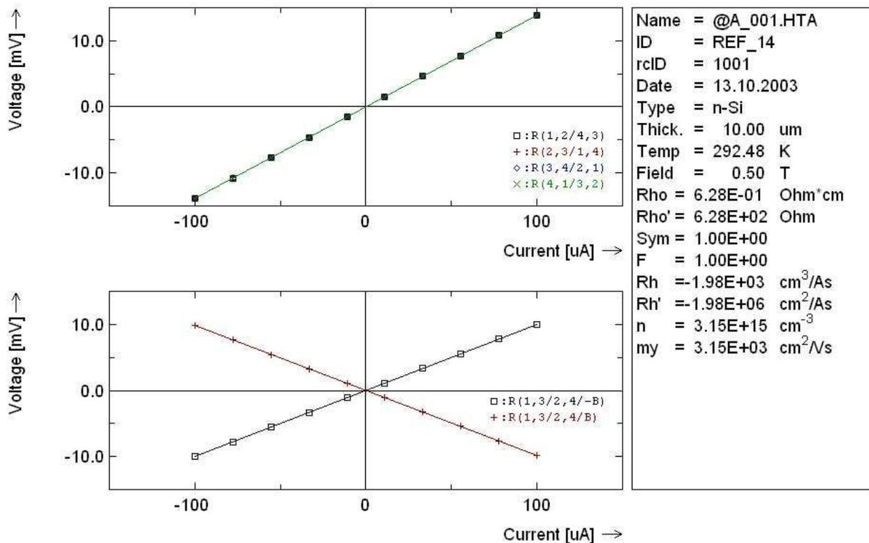
A complete sample characterization including all 2-point, all 4-point, v.d. Pauw and Hall measurements are shown in the last two pages. The plots are as printed from our software. The first page shows a measurement @ two magnetic fields, the second one a measurement under varied magnetic field.
