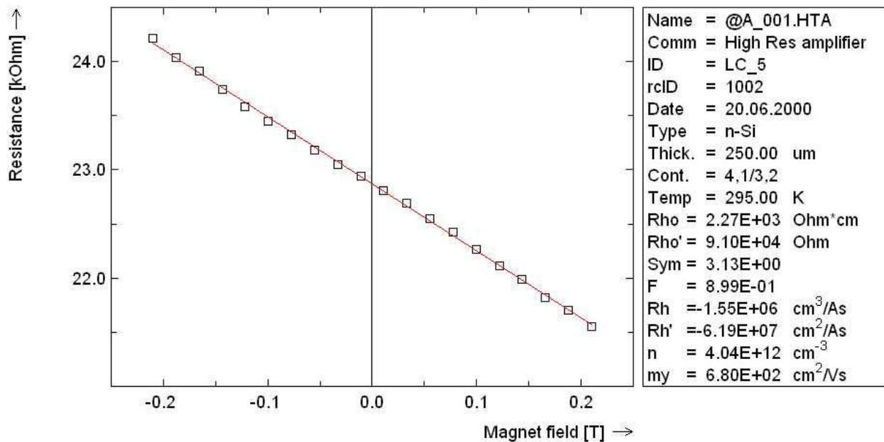
Each Hall resistance in the plot above is still measured by an V/I curve and calculated by automatic regression.
